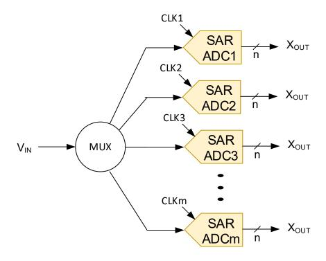
Time interleaving increases effective conversion rate by factor of m
