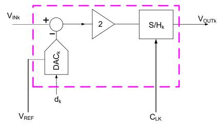
$$V_{O} = \begin{cases} 2V_{IN} + \frac{V_{REF}}{2} & V_{IN} < 0 \\ 2V_{IN} - \frac{V_{REF}}{2} & V_{IN} > 0 \end{cases}$$
