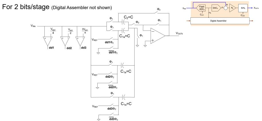
$$V_{\text{out}} = V_{\text{IN}} \left( 1 + \frac{C_{_{1a}} + C_{_{1b}} + C_{_{1c}}}{C_{_{2}}} \right) - \left( d_{_{d1}} \left( \frac{C_{_{1a}}}{C_{_{2}}} \right) + d_{_{d2}} \left( \frac{C_{_{1b}}}{C_{_{2}}} \right) + d_{_{d3}} \left( \frac{C_{_{1c}}}{C_{_{2}}} \right) \right) V_{\text{REF}}$$
